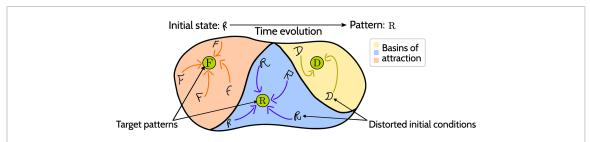
**Figure 1.** The phase space of a classical system powered with AM capabilities can be divided into different regions called basins of attraction. Each basin contains a stable fixed point of the dynamics, which is regarded as the pattern or memory. Then, any other initial condition belonging to the same basin will naturally converge to the corresponding pattern. Thus, the initial corrupted or distorted state is associated with the corrected version of the state, the pattern.
